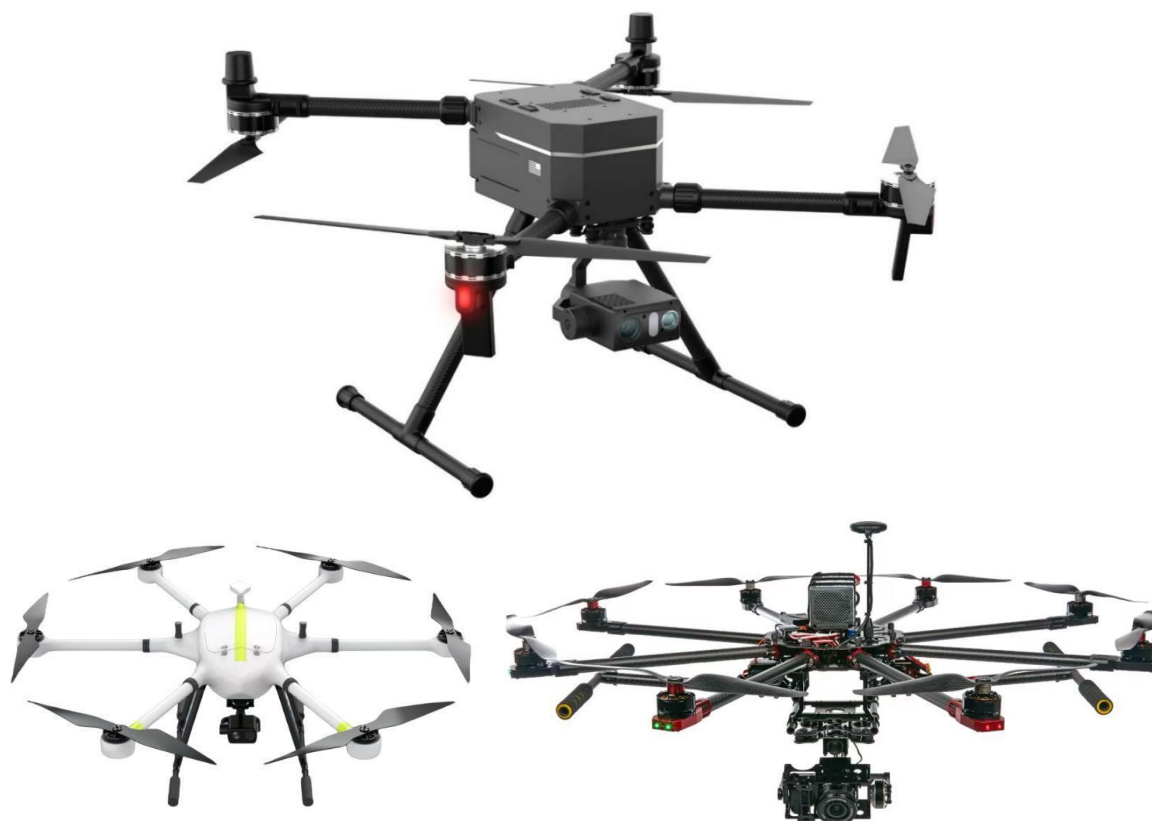
Obr. 6: Typy Quadkoptéry (nahore), hexakoptera (vlevo dole) a Oktokoptera (vpravo dole). Zdroj: Quadcoptera: Autonomous Drones For Mission-Critical Applications | Flyby Robotics Hexacoptera: UnmannedRC 1600 Hexacopter for Heavy Lifting 10KG 55MINS
