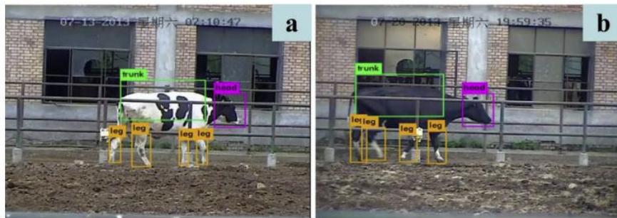
Fig. 2 – YOLOv3 algorithm detection results (a) blocked by a small near-view object
